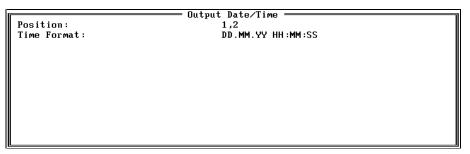
Do not make any changes in this window and press the **F4 Accept** function key. The Date/Time field will be displayed in the start-up picture:
